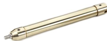
The **COA series** is part of the nautical standard Grices production. The usage of **AISI 316** stainless steel and OT58 brass assures the total absence of corrosion. The sleek and smooth design makes this series suitable for nautical applications in particular for ramp movement and gangway extraction, with continuous nominal pressure up to **8 MPa**.
